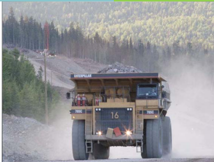
7 - Haul trucks also transport waste rock from a blast out of the pit to a waste rock dump.
