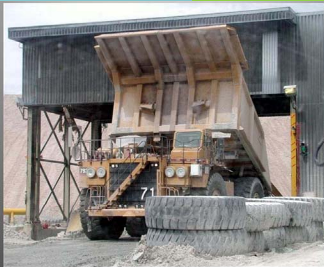
6 - There are different styles of primary crushers (e.g. jaw, gyratory, cone) which all use heavy steel parts that move together to break up the rock. Crushed ore must be hauled by truck or conveyed to a mill for further processing.
