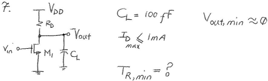
$$I_{D, max} = \frac{V_{DD} - V_{out, min}}{R_D}$$
