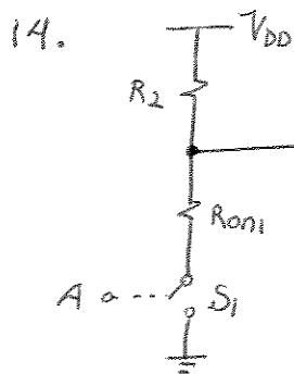
$$R_{on1} \ll R_2 \rightarrow V_{out, min} \approx 0$$
