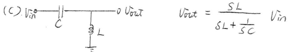
$$\frac{V_{\text{out}}}{V_{\text{in}}} = \frac{s^2 LC}{s^2 + \frac{1}{LC}} \quad \text{zeros: Two zeros at } 0; \quad \text{poles} = \pm i \frac{1}{\sqrt{LC}}$$
