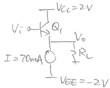
$$45. P_{R_L} = \frac{V_P^2}{2R_L} = \frac{(V_{CC} - V_{BE})^2}{2R_L}$$
