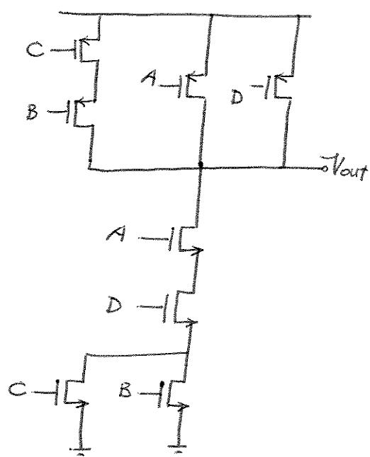
$$V_{out} = \overline{(B+C)D.A}$$
