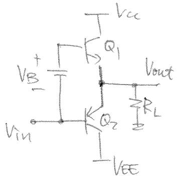
$$V_{out} = V_{in} + |V_{BEz}|$$
