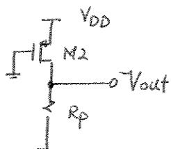
$$I_{D2} = \frac{1}{2} \mu_P C_{ox} \left(\frac{W}{L}\right)_2 \left[ 2(V_{DD} - |V_{TH2}|)(V_{DD} - V_{out}) - (V_{DD} - V_{out})^2 \right]$$
