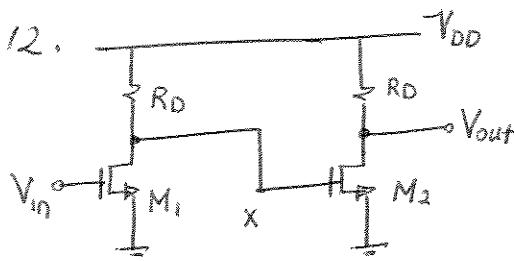
The small signal gain of the circuit is equal to  $-g_m R_D$  and since
