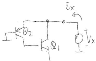
$$\begin{aligned} \bar{i}_x &= \bar{i}_{e2} + \bar{i}_{c1} \\ &= \bar{i}_{e2} + \bar{i}_{b1} \beta_1 \\ &= \bar{i}_{e2} + \bar{i}_{c2} \beta_1 \\ &= \bar{i}_{c2} + \bar{i}_{b2} + \bar{i}_{c2} \beta_1 \\ &= \bar{i}_{c2} \left(1 + \beta_1 + \frac{1}{\beta_1}\right) \\ &= V_x g_{m2} \left(1 + \beta_1 + \frac{1}{\beta_1}\right) \end{aligned}$$
