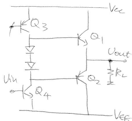
$$P_{Q_1, \text{MAX}} = V_{CE} \times I_{C_1, \text{MAX}} = (V_{CC} - V_{out}) I_{C_1, \text{MAX}}$$
