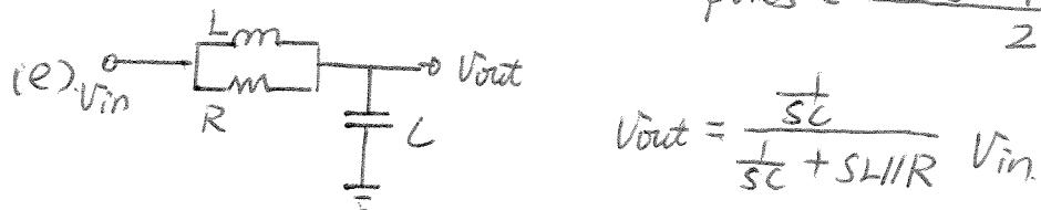
$$\frac{V_{\text{out}}}{V_{\text{in}}} = \frac{\frac{1}{RC}(s + \frac{R}{L})}{s^2 + \frac{s}{RC} + \frac{1}{LC}}, \quad \text{zero} = -\frac{R}{L}; \quad \text{poles} = \frac{-\frac{1}{RC} \pm \sqrt{(\frac{1}{RC})^2 - \frac{4}{LC}}}{2}$$
