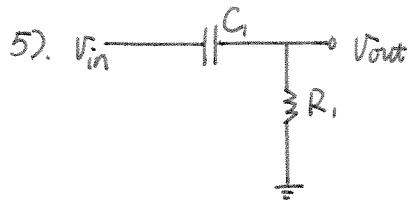
$$\frac{V_{out}}{V_{in}} = \frac{R_1}{R_1 + \frac{1}{Cs}} = \frac{\frac{1}{s}}{s + \frac{1}{R_1 C_1}}$$
