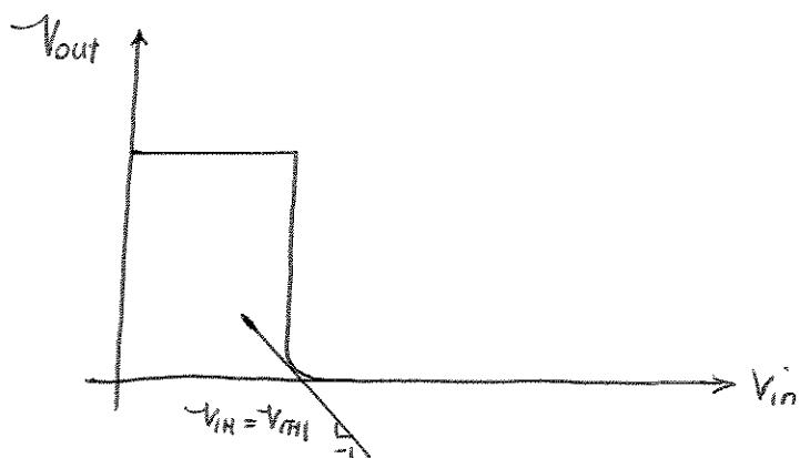
Note that the separation between  $V_{IH}$  and  $V_{IL}$  depends on the slope of VTC in the transition region. If "a" approaches either "0" or infinity, VTC exhibits infinite gain in its transition region. Therefore  $V_{IL}$  and  $V_{IH}$  coincide.
