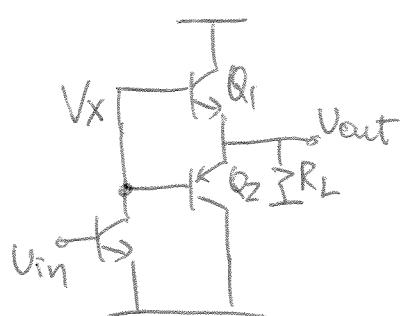
$$A_V = \frac{V_{out}}{V_x} \cdot \frac{V_x}{V_{in}}$$
