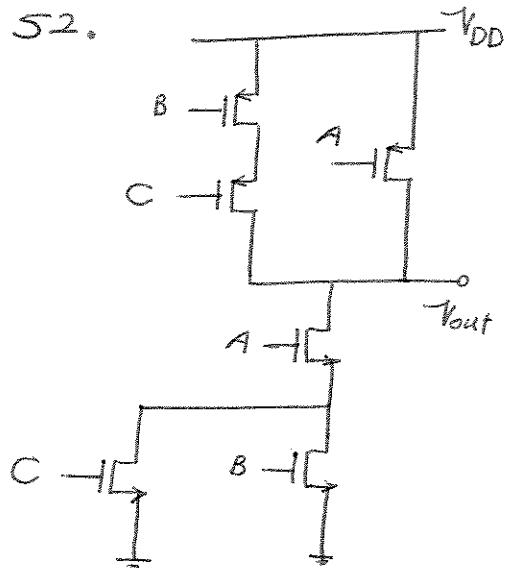
$$V_{out} = \overline{(B+C)A}$$
