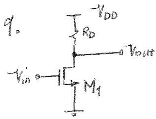
Small signal gain of the inverter is equal to  $-g_m R_D$
