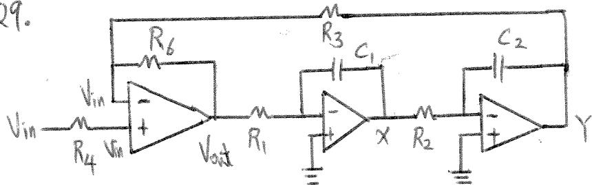
$$V_x = -\frac{V_{out}}{R_1} \left( \frac{1}{C_1 s} \right), \quad V_y = -\frac{V_x}{R_2} \left( \frac{1}{C_2 s} \right), \quad V_{out} = V_{in} - \frac{(V_y - V_{in}) R_6}{R_3}$$
