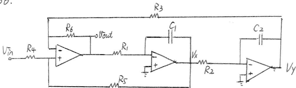
$$\text{Low pass, } \frac{V_y}{V_{in}} = \frac{\alpha s^2}{s^2 + \frac{w_h}{\alpha} s + w_h^2} \cdot \frac{1}{R_1 R_2 C_1 C_2 s^2}$$
