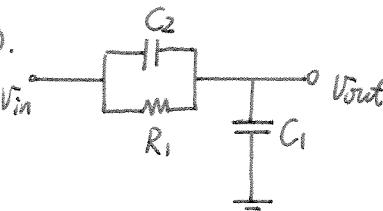
$$\frac{V_{out}}{V_{in}} = \frac{\frac{1}{Cs}}{\frac{1}{Cs} + R_1 // sC_2}$$
