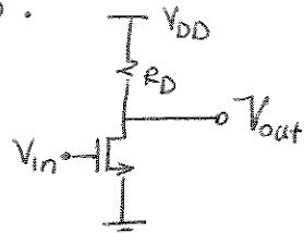
$$V_{OL} = 100mV \quad P_{av} = 0.25mW$$
