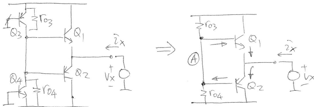
$$v_{eb} = v_x \frac{(r_{\pi_1} \parallel r_{\pi_2})}{(r_{\pi_1} \parallel r_{\pi_2}) + (r_{03} \parallel r_{04})}$$
