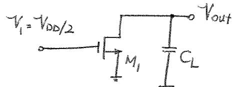
$$V_{DD}/2 - V_{TH1} < V_{out} < V_{DD} \quad M_1 \text{ in saturation}$$
