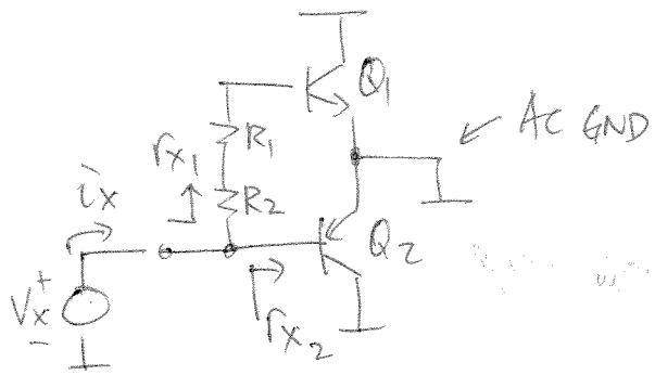
$$R_{in} = \frac{V_x}{i_x} = R_{x_1} \parallel R_{x_2}$$
