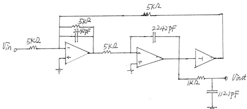
$R_1 = R_2 = R_4$  to match low frequency gain requirement.
