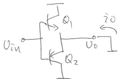
$$g_m = \frac{i_o}{v_{in}} = -(g_{m1} + g_{m2})$$
