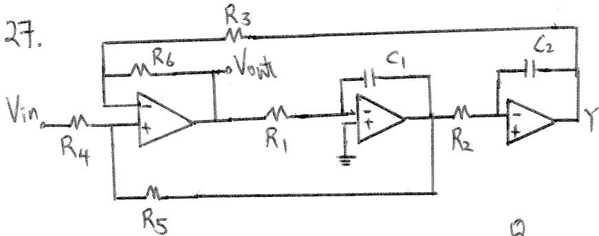
Low Pass, low freq gain of 2.  $S_{R_3, R_6}^Q = 0$
