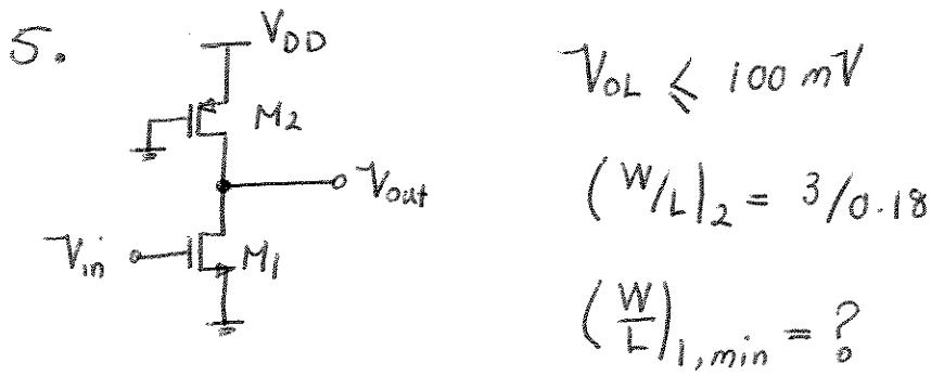
$V_{in} = V_{DD} \rightarrow M_1$  operates in the triode region and  $M_2$  in the saturation.
