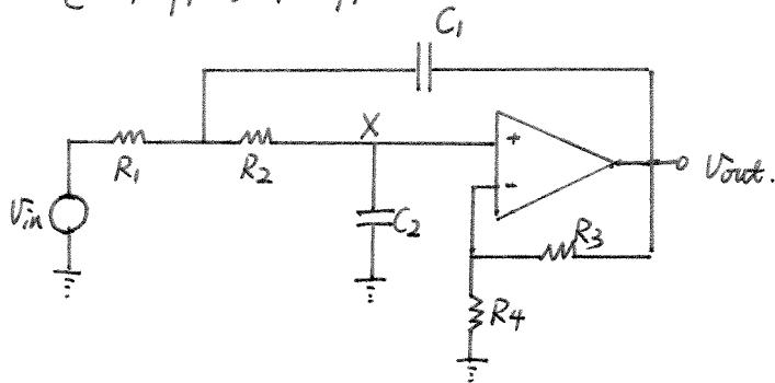
$$\frac{V_{out}}{V_{in}} = \frac{1 + \frac{R_3}{R_4}}{R_1 R_2 C_1 C_2 S^2 + (R_1 C_2 + R_2 C_2 - R_1 \frac{R_3}{R_4} C_1)S + 1}$$
