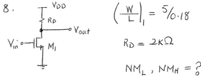
Small signal gain of the circuit is equal to  $-g_m R_D$
