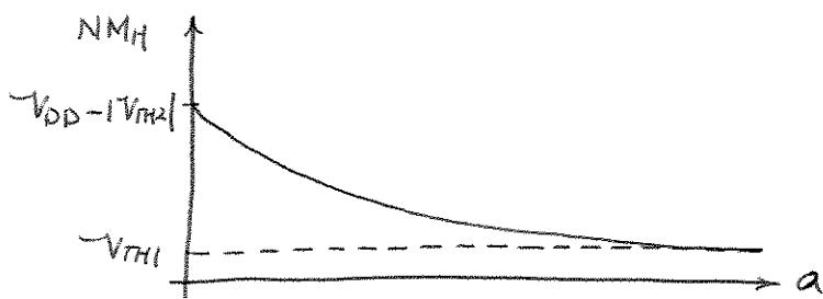
If  $a = \frac{\mu_n}{\mu_p} \times \frac{(\frac{W}{L})_1}{(\frac{W}{L})_2} \rightarrow 0$ , it implies that PMOS transistor is much stronger than NMOS. Therefore, as  $V_{in}$  increases from 0V, the output of inverter remains at  $V_{DD}$  until input reaches  $V_{DD} - |V_{TH2}|$ .
