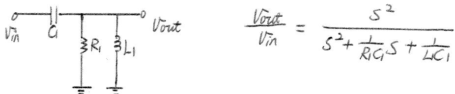
$$\frac{V_{out}}{V_{in}} = \frac{s^2}{s^2 + \frac{1}{R_1 C_1} s + \frac{1}{L_1 C_1}}$$
