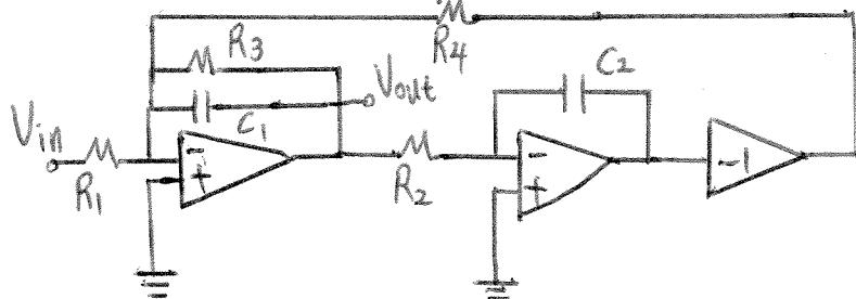
$$\omega_n = \frac{1}{\sqrt{R_2 R_4 C_1 C_2}}, \quad Q^{-1} = \frac{1}{R_3} \sqrt{\frac{R_2 R_4 C_2}{C_1}}$$
