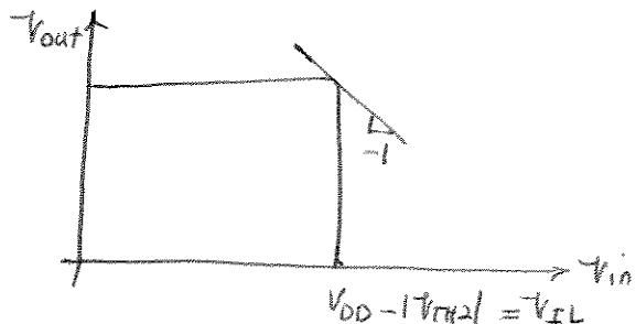
When  $a \rightarrow \infty$ , NMOS is prevailing and once input voltage hits the threshold voltage of NMOS, output voltage falls sharply to 0V.
