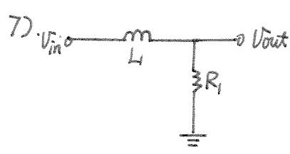
$$\frac{V_{\text{out}}}{V_{\text{in}}} = \frac{R_1}{R_1 + L_1 s} = \frac{R_1/L_1}{s + R_1/L_1}$$
