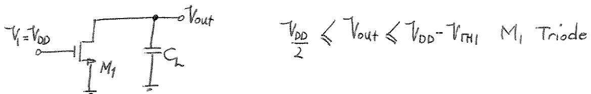
$$C_L \frac{dV_{out}}{dt} = -I_{D1} = -\frac{1}{2} \mu_n C_{ox} \left( \frac{W}{L} \right)_1 (V_{DD} - V_{TH1})^2 = -\frac{1}{2} \times 100 \times 10^{-6} \times \frac{1}{0.18} (1.8 - 0.4)^2 = 5.44 \times 10^{-4} \text{ A}$$
