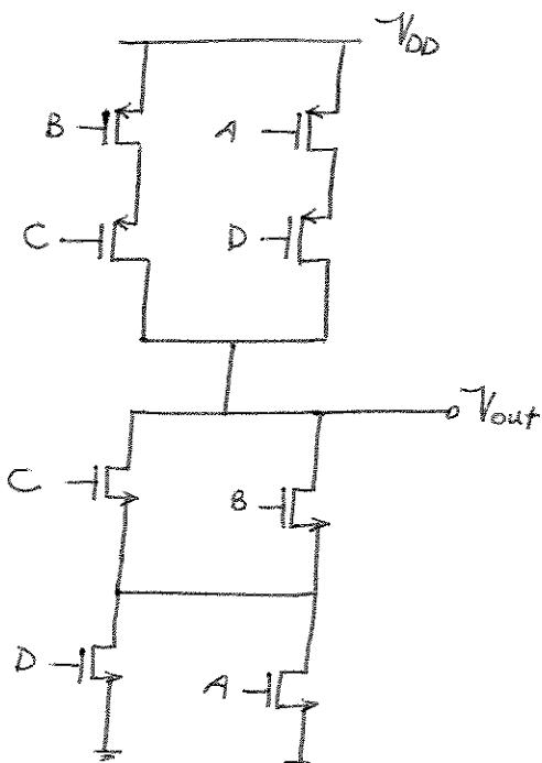
$$V_{out} = \overline{(A+D) \cdot (B+C)}$$
