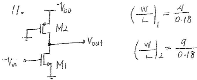
To calculate  $V_{IL}$ , we assume that  $M_1$  and  $M_2$  operate in saturation and triode region respectively.
