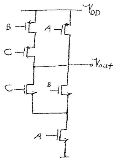
$$V_{out} = \overline{(B+C).A}$$
