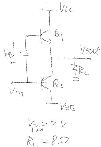
$$\begin{aligned}\hat{I}_o &= -g_{m1} V_i + (-V_i) g_{m2} \\ &= -(g_{m1} + g_{m2}) V_i\end{aligned}$$
