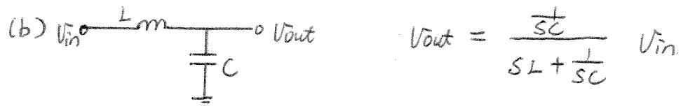
$$\frac{V_{\text{out}}}{V_{\text{in}}} = \frac{1/(LC)}{s^2 + \frac{1}{LC}} \quad \text{zero: No finite zero; poles} = \pm i \frac{1}{\sqrt{LC}}$$
