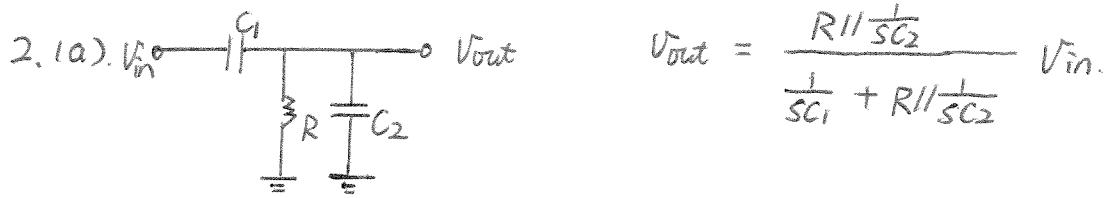
$$\frac{V_{\text{out}}}{V_{\text{in}}} = \frac{\frac{1}{s(C_1+C_2)}}{s + \frac{1}{R(C_1+C_2)}} , \quad \text{zero} = 0; \quad \text{pole} = -\frac{1}{R(C_1+C_2)}$$
