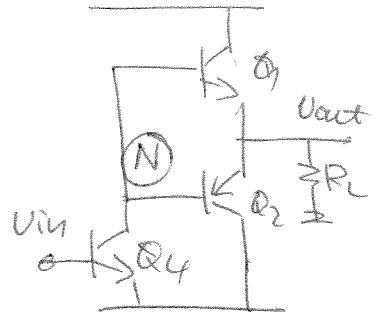
$$\Rightarrow \frac{V_{out}}{V_{in}} = +g_{m4} (r_{\pi1} \parallel r_{\pi2}) (g_{m1} + g_{m2}) R_L = 5$$
