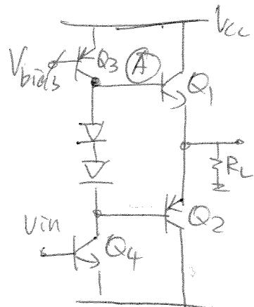
$$(c) P_{AV} = \frac{V_P}{R_L} \left( \frac{V_{CC}}{\pi} - \frac{V_P}{4} \right)$$
