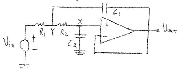
$$H(s) = \frac{1}{R_1 R_2 C_1 C_2 s^2 + (R_1 + R_2) C_2 s + 1}, \quad Q = \frac{1}{R_1 + R_2} \sqrt{\frac{R_1 R_2 C_1}{C_2}},$$
