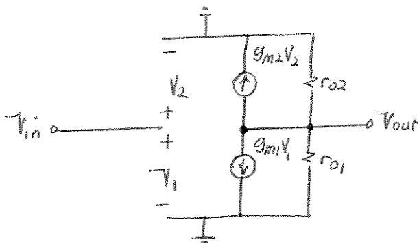
$$V_{out} = (-g_{m1}V_1 - g_{m2}V_2) / (r_{o1} \parallel r_{o2})$$
