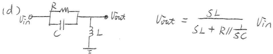
$$\frac{V_{\text{out}}}{V_{\text{in}}} = \frac{s(s + \frac{1}{RC})(RC)^2}{s^2 + \frac{s}{RC} + \frac{1}{LC}} \quad \text{zeros: } 0, -\frac{1}{RC}$$
