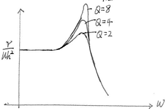
$$13). \quad H(s) = \frac{\beta s}{s^2 + \frac{w_n}{\alpha} s + w_n^2}, \quad H(jw) = \frac{j\beta w}{w_n^2 + j\frac{w_n}{\alpha} w - w^2}$$
