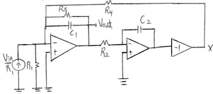
When  $R_1$  and  $V_{in}$  are replaced with its Norton equivalent, we see that the "upper" terminal of  $R_1$  is at virtual ground. Since  $R_1$ 's two terminals are at the same potential, no current will flow through it, therefore it can be seen as an open. So  $R_1$  is not in the signal path, and therefore will not affect the frequency response. However, since its magnitude is embedded in the Norton current source, it will affect the DC gain.
