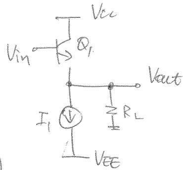
$$(b) \text{ When } V_{out} = V_P, \quad I_{C_1} = I_I + \frac{V_{out}}{R_L} = \frac{V_P}{R_L} + \frac{V_P}{R_L}$$
