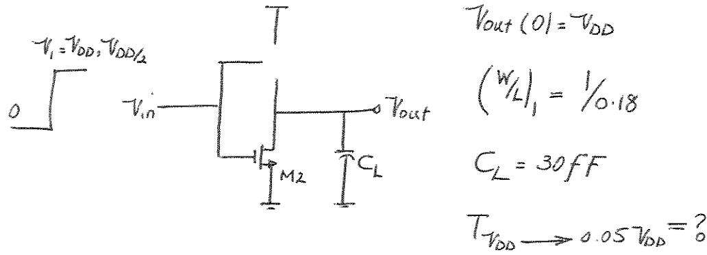
$$(a) V_i = V_{DD} \quad V_{DD} - V_{TH1} < V_{out} < V_{DD} \quad M_1 \text{ in Saturation}$$
