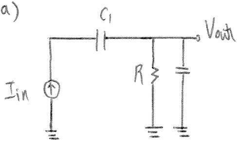
$$\frac{V_{out}}{I_{in}} = \frac{1/C_2}{S + 1/(RC_2)}$$
