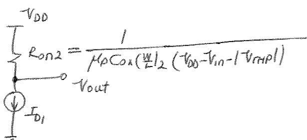
By increasing  $L_2$ ,  $R_{on2}$  becomes larger; as a result, lower value of  $I_{D1}$  causes comparable voltage drop at the output. This will drive  $M_2$  into the saturation with lower current ( $I_{D2}$ ) and, hence, lower value of  $V_{in}$ . Therefore, characteristic is shifted to the left and small signal gain will be higher.
