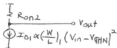
By increasing  $L_1$ ,  $I_{D1}$  is weakened due to the inverse proportionality; as a result, an excess  $V_{in}$  is required to drop  $V_{out}$  to the point where  $V_{out} = V_{in} + |V_{TH2}|$  and  $M_2$  is placed at the edge of saturation.
