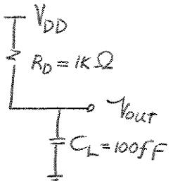
$$V_{R_D} = (V_{DD} - V_{out})$$
