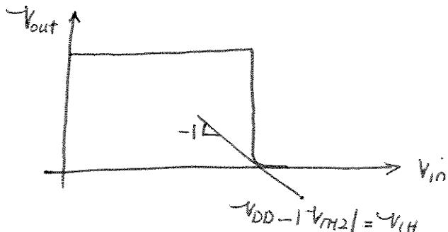
When "a" approaches infinity, NMOS is prevailing and once input voltage hits the threshold voltage of NMOS, output voltage falls sharply to 0V.
