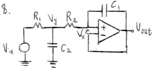
Assuming an ideal Op-amp,  $V_x = V_{out}$ . Therefore, no current will flow thru  $C_1$ . Moreover, since the input impedance of an Op-amp ( $Z_{ideal}$ ) is infinite, no current will flow thru  $R_2$  as well, which means  $V_y = V_x = V_{out}$ .
