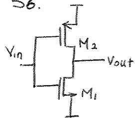
$$V_{in} = V_{out} = 0.8 \text{ V}, I_{D1} = I_{D2} = 0.5 \text{ mA}$$
