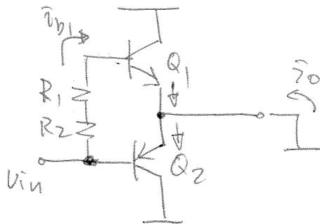
$$\bar{i}_o = -g_{m1}U_{be1} + g_{m2}|U_{be2}| \quad (\bar{i}_o = \bar{i}_{c2} - \bar{i}_{c1})$$
