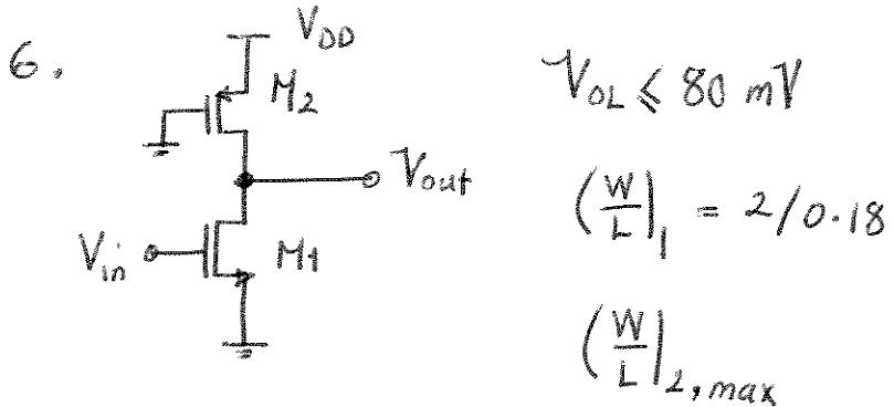
$V_{in} = V_{DD} \rightarrow M_1$  operates in the triode region and  $M_2$  in the saturation
