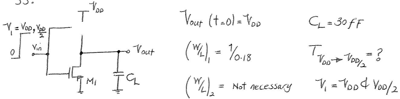
$$(a) \quad V_i = V_{DD} \quad V_{DD} - V_{TH1} \leq V_{out} \leq V_{DD} \quad M_1 \text{ saturation}$$
