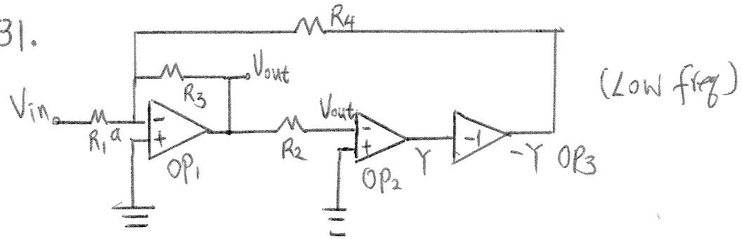
$V_{out}$  equals zero because of  $OP_2$ 's negative feedback.
