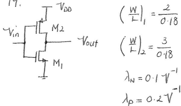
Replacing M<sub>1</sub> and M<sub>2</sub> with their small-signal model in the saturation region yields:
