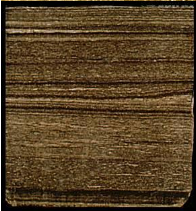
Microfractures in organic rich shale. Hunt, 1995.
