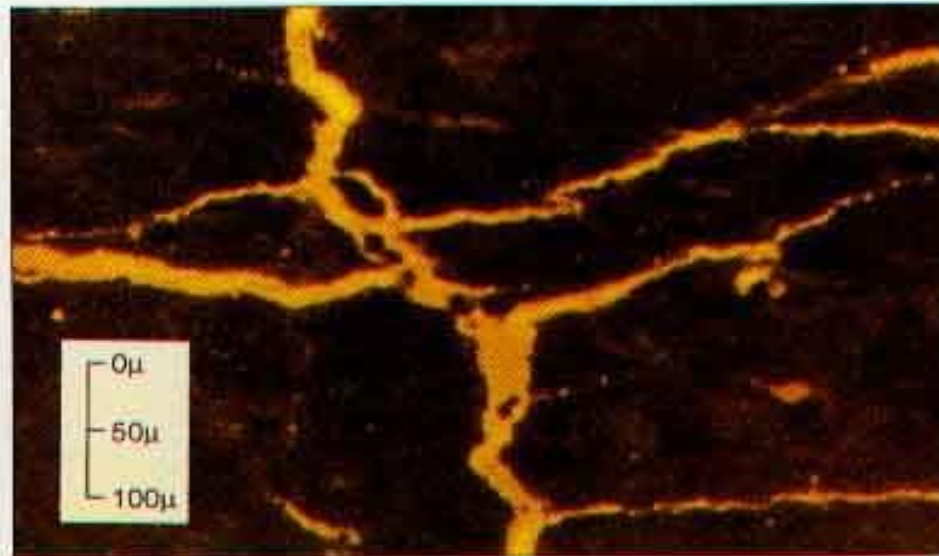
Microfractures in organic rich shale. Hunt, 1995.
