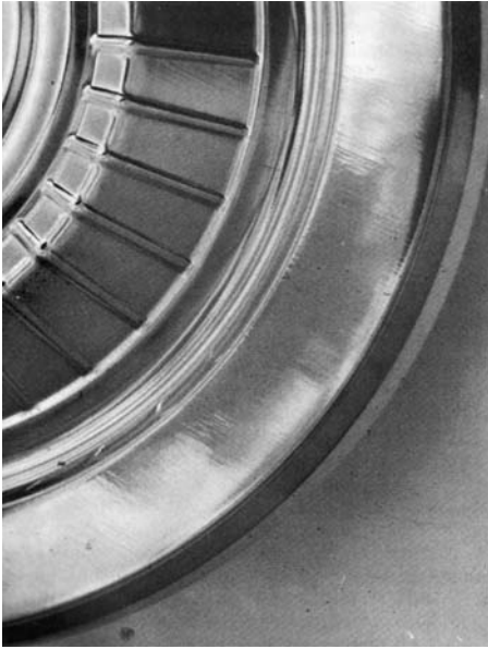
19.2. Ridging in a 430 stainless steel. From Making, Shaping and Treating of Steel , 9th ed. (United States Steel Corporation, 1971), p. 1180.
