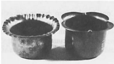
14.3. Wrinkling of partially drawn cups due to insufficient hold-down. From D. J. Meuleman, op. cit.
