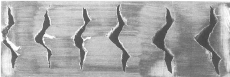
10.16. Cracks formed in a molybdenum bar during rolling under high \Delta conditions.
