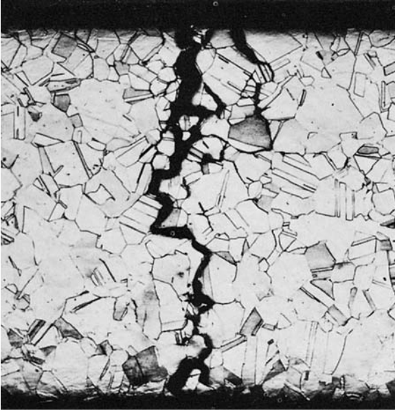
19.16. Stress-corrosion cracking in brass. From Metals Handbook , 8th ed., Vol. 7 (ASM, 1972), p. 291.
