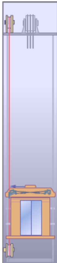
2. The governor locks and activates the pull rods.
