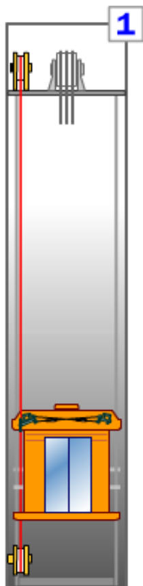
1. If the elevator falls the governor is activated.
