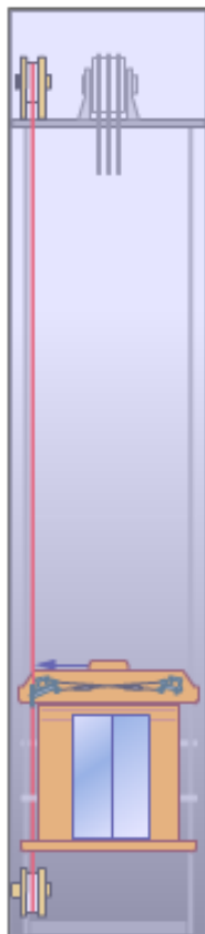
2. The governor locks and activates the pull rods.
