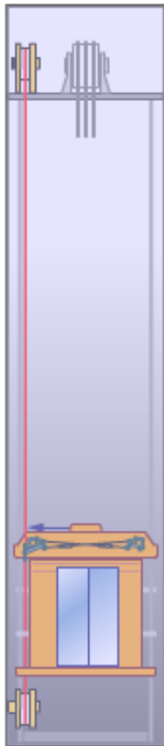
3. The pull rods engage the safety brakes.
